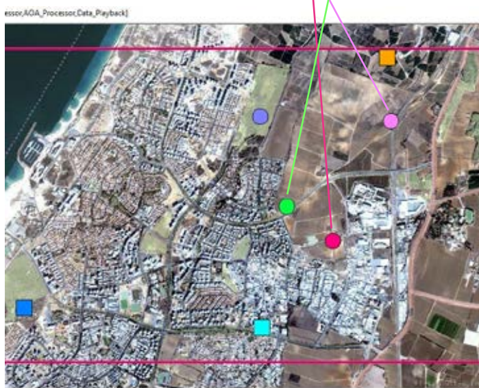
<< Figure 24: Receiver and transmitter setup including a frequency hopping transmitter
