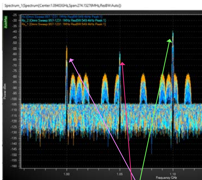
<< Figure 23: Spectrum with frequency hopping signal
