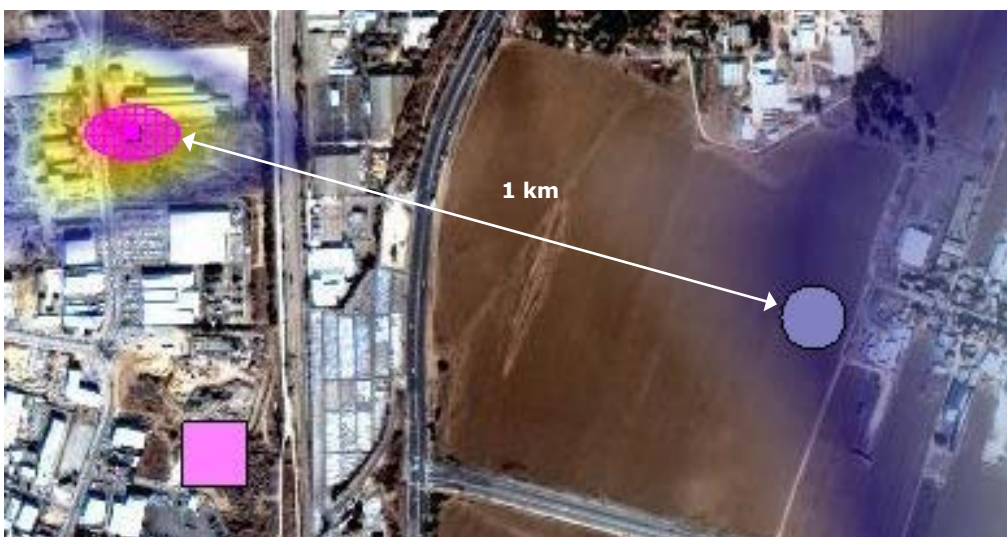
<< Figure 4: POA performance for distant CW Tx, large geolocation error with unstable reading
