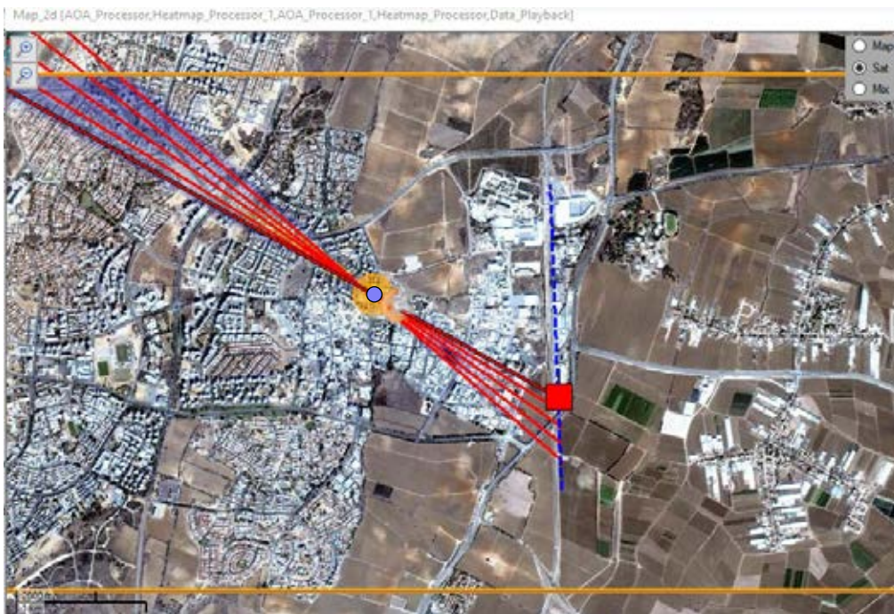
<< Figure 15: Cumulative AOA tracking, 1 GHz PSK transmitter located to a precision of 117 m by 78 m using a single moving antenna array.
