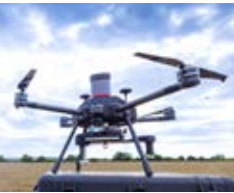
Tethered drone Bespoke ISS Sensus M4 with dual sensor payloads
