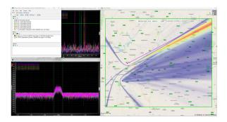
The software uses 3D TDoA to detect the signal at an altitude of approximately 2km and a distance of approximately 50km (26 miles) from the closest RFeye Node.
