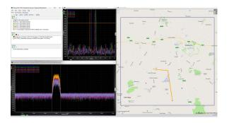
The software uses 3D TDoA to detect the signal approaching the sensor network and then tracks it as it flies. The signal is approximately at an altitude of 100 meters.
