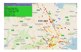
This detector-based solution is designed to automatically detect and geolocate specific signals (ADS-B in this case) each time they are received by the sensor network. CRFS' RFeye software supports detector-based 3D TDoA, triggering signal detection and geolocation workflows the moment a matched signal is identified.
